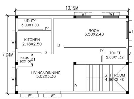
PROPOSED TYPICAL GROUND, FIRST & SECOND FLOOR PLAN
